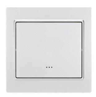
Wireless repeater • Voltage: 230 V AC, 50 Hz • Maximum charges: 6A (1380W) • Range up to 30m(straight line) • Dimensions: 86x86x47mm
