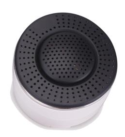
Volume: 80-110dB • Current: DC 5V / 1A • Range up to 30m (straight line) • Operating temperature: -10°C up to 50°C • Operating humidity: <80%
